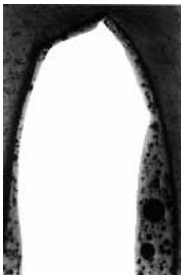
Direct-on white enamelling on a squeezed-off edge (50 : 1)
